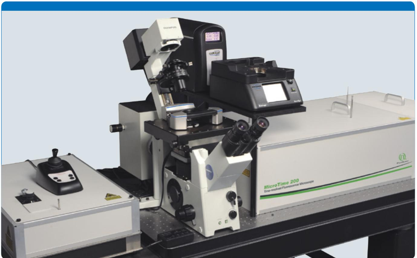
Figure 1. Combined setup of the BioScope Catalyst and the MicroTime 200. The AFM with its sample stage is mounted on the inverted microscope body of the MicroTime 200, which is configured for objective scanning.
