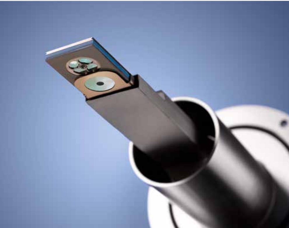
QUANTAX FlatQUAD is the EDS microanalysis system based on the revolutionary XFlash® FlatQUAD. This special annular four-channel silicon drift detector is inserted between SEM pole piece and sample, achieving maximum solid angle in EDS. In combination with the ESPRIT analytical software suite QUANTAX FlatQUAD provides previously unheard of mapping performance, even for the most difficult samples.
