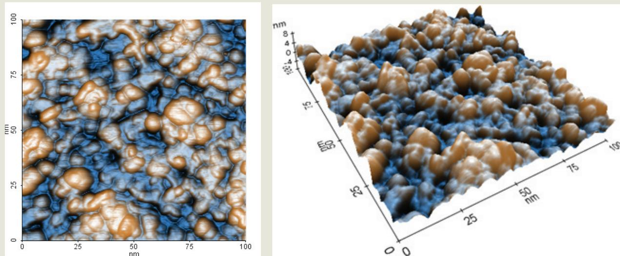
Figure 2. High resolution (100 nm x 100 nm) image of a gold surface, acquired by True Non-Contact Mode of the XE-100 AFM.
