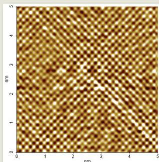
Figure 1. HOPG image taken with XE-100 (5 nm x 5 nm scan size). This image shows atomic lattice, not individual atoms.
